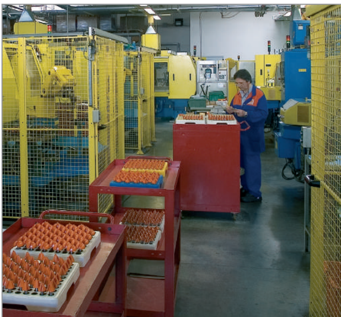
Loading the automated multi-axis CNC sharpening machines.
